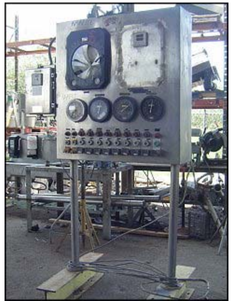
Control Panel with a small Pro Controls Inc. evaporator steam controller. Serial no. 96134. 120 V, 15 A, 1 Phase. Taylor chart recorder, S/N: 122RV168-2617. Chart or scale: OP 534. Primary range (red) 120, 230 degrees F. Overall dimensions: 4 ft. 3-1/2 in. L. x 3 ft. 2-1/8 in. W. x 7 ft. 3 in. H.
