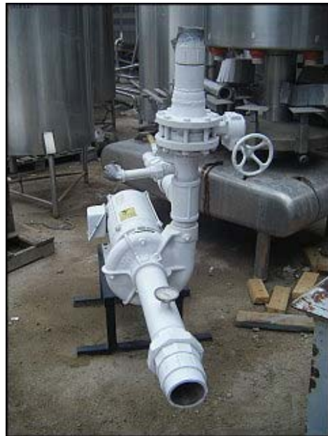
(1) Berkeley Centrifugal Pump. Model no. B3ZPLS. (1) temperature gauge. Motor specifications: 20 hp, 3470 rpm, 230/460 V, 47/23.5 A, 60 Hz, 3 Phase. Inlets/Outlets: (1) 4 in. MNPT. (1) 3 in. FNPT. (1) 1-1/4 in. MNPT. (1) 2 in. shut on/off valve. Overall dimensions: 4 ft. 3-3/4 in. L. x 2 ft. W. 4 ft. 5-5/8 in. H.
