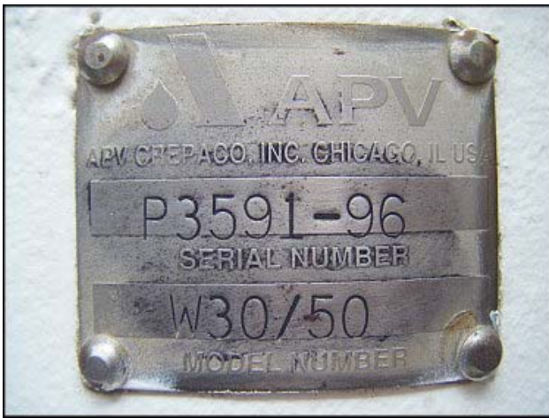
(1) APV Centrifugal Pump. Model no. W30/50. Serial no. P3592-96. U.S. Electrical motor: 3 hp, 1750 rpm, 230/460 V, 8.8/4.4 A, 60 Hz, 3 phase. Inlets: (1) 3 in. S-line. Outlets: (1) 2-1/2 in. S-line. Overall dimensions: 1 ft. 9-1/2 in. L. x 1 ft. 5/8 in. W. x 1 ft. 3-7/8 in. H.
