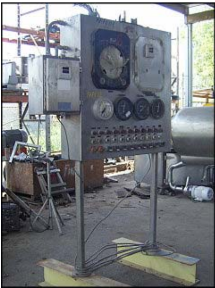
Control Panel with a small Pro Controls Inc. evaporator steam controller. Serial no. 96134. 120 V, 15 A, 1 Phase. Taylor chart recorder, S/N: 122RV168-2617. Chart or scale: OP 534. Primary range (red) 120, 230 degrees F. Overall dimensions: 4 ft. 3-1/2 in. L. x 3 ft. 2-1/8 in. W. x 7 ft. 3 in. H.
