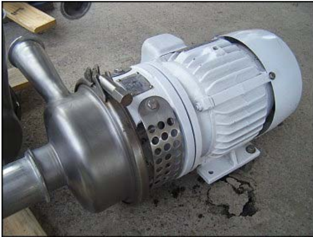
(1) APV Centrifugal Pump. Model no. W30/50. Serial no. P3592-96. U.S. Electrical motor: 3 hp, 1750 rpm, 230/460 V, 8.8/4.4 A, 60 Hz, 3 phase. Inlets: (1) 3 in. S-line. Outlets: (1) 2-1/2 in. S-line. Overall dimensions: 1 ft. 9-1/2 in. L. x 1 ft. 5/8 in. W. x 1 ft. 3-7/8 in. H.
