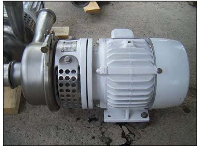
(1) APV Centrifugal Pump. Model no. W30/50. Serial no. P3592-96. U.S. Electrical motor: 3 hp, 1750 rpm, 230/460 V, 8.8/4.4 A, 60 Hz, 3 phase. Inlets: (1) 3 in. S-line. Outlets: (1) 2-1/2 in. S-line. Overall dimensions: 1 ft. 9-1/2 in. L. x 1 ft. 5/8 in. W. x 1 ft. 3-7/8 in. H.
